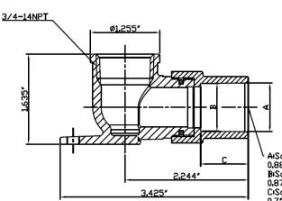
AiSocket Entrance Diameter 0.884\*±0.003 BiSocket Bottom Diameter 0.870\*±0.003\* CiSocket Length 0,7\* min
