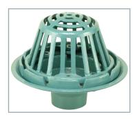
10" Diameter Roof Drain, Epoxy Coated Cast Iron Body, Bolt Down Gravel Guard, and Epoxy Coated Metal Dome.
