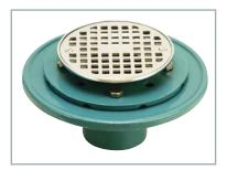
Heavy Duty Epoxy Coated Cast Iron Body, Epoxy Coated Bolt Down Ring, and Adjustable Cast Brass Strainer Assembly Chrome Plated or Polished Brass.
